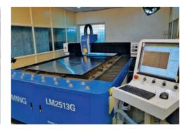
CNC Laser cutting machine is used for marking and cutting of stainless steel sheets. Using this machine very accurate cutting and punching of the sheets is attained which will gives us the precise assembling of the machine and thus improving the overall performance of the machine.
